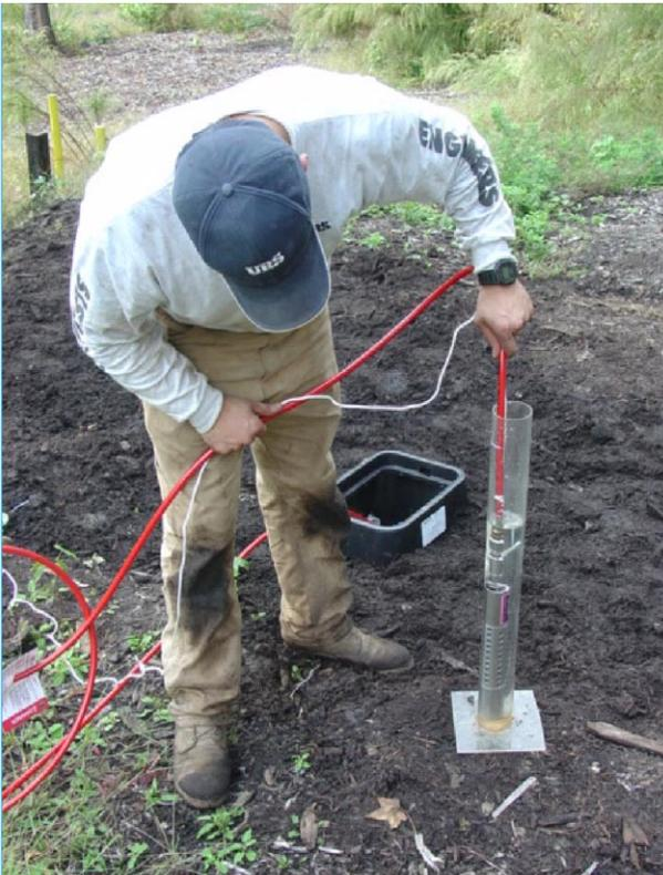
Testing an iSOC infusion device for hydrogen delivery.
