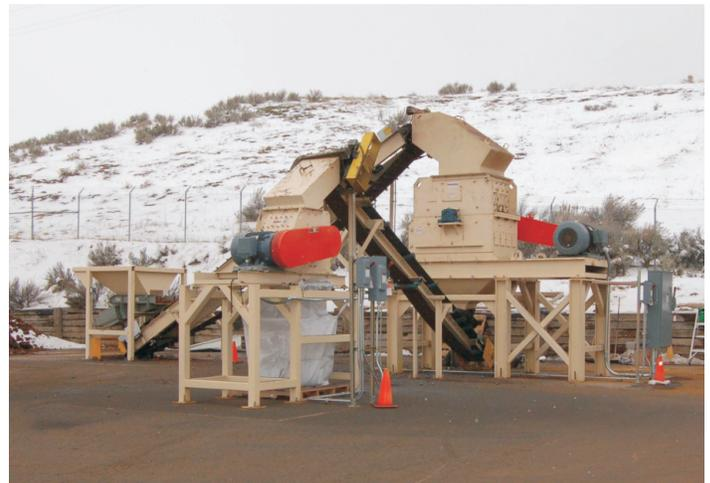
This hammermill crushed cast-iron dummy bombs collected from the Utah Test and Training Range for use as reactive agent for Permeable Reactive Barriers.
