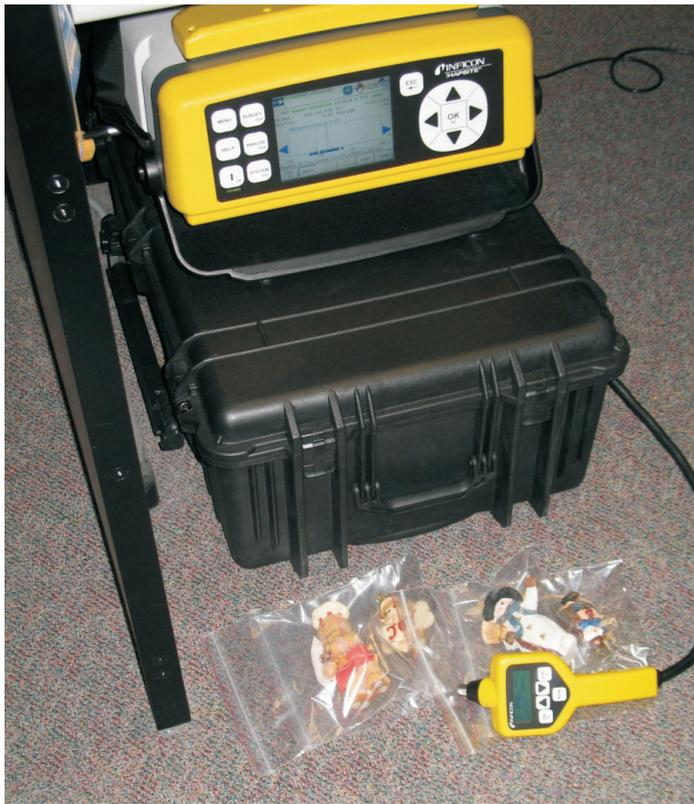
The Hazardous Air Pollutants on Site, or HAPSITE, is a portable vapor analyzer capable of finding individual objects
