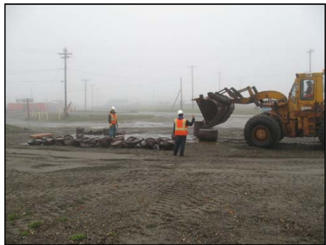
Photo 5. Eric Jenks (left), Mike Flisk (center), and Dave Vandergriff (right) are processing drums in the village of Kaktovik, Alaska. The drums are cleaned and crushed before being placed in a container for shipment to a metal recycler in Fairbanks, Alaska.
