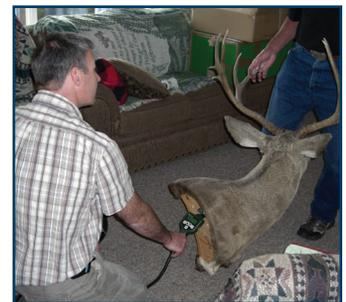
Using a device known as a HAPSITE, Hill workers identify this stuffed deer head as the source of VOC vapors in a home. If VOC vapors can be traced to an inside source, it saves the Air Force thousands of dollars that would have otherwise been spent installing and maintaining a vapor mitigation system.
