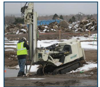
Using the membrane interface probe (MIP) on a direct push rig. This device is able to characterize soil type and screen for the presence of Volatile Organic Compounds in real time. This approach allowed a 12.5 acre site to be characterized in little time and minimized the amount of soil needing removal.
