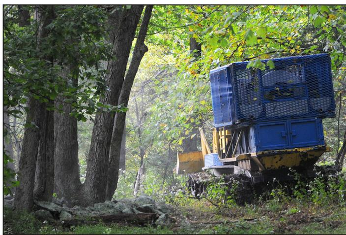
Forest wide herbicide application using a modified skidder. Note the nozzles blasting herbicide mist from the back sides of the skidder.
