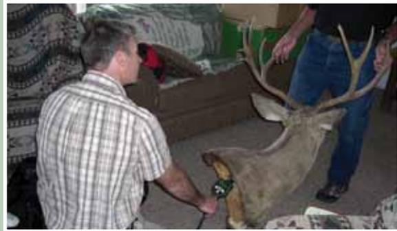
*Using a device known as a HAPSITE, Hill AFB workers identify this stuffed deer head as the source of volatile organic compound (VOC) vapors in a home. If the Air Force can trace VOC vapors to an inside source, it saves them thousands of dollars that would have otherwise been spent installing and maintaining a vapor mitigation system.*
