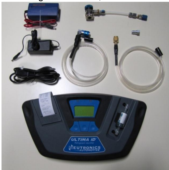
Photo 4 - Pictured is the refrigerant identifier test kit, including adapters, needed for common A/C service connections.
