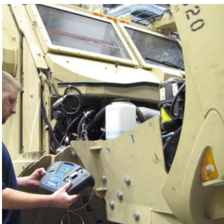
Photo 6 – Tester being used on a tactical vehicle to analyze refrigerant purity.
