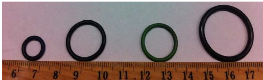
Photo 2 – Air conditioning o-ring seals new on left; exposed to counterfeit refrigerant on right.
