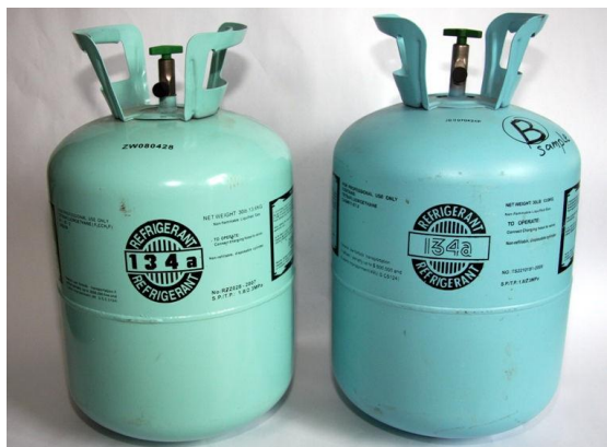
Photo 1 - Counterfeit refrigerant cylinder (left); legitimate refrigerant cylinder from reputable company (right).
