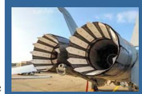
Figure 4: VEN Chevrons Installed on Engine
