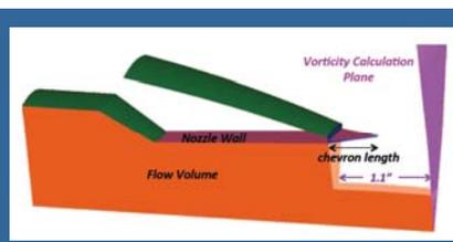
Figure 6: Illustration of the Chevron Extension to the Faceted Nozzle
