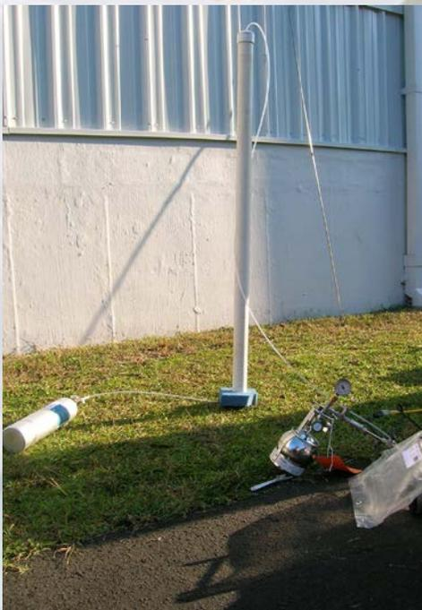
*Suma Canisters collect Soil-Vapor Samples during Phase 2 of the VI Investigation*
