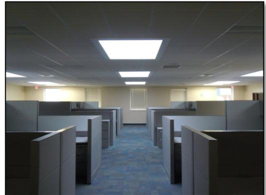
*Building 454 is one of the “greenest” buildings on the installation and has a motion-sensitive lighting system to turn on and off lights.*
