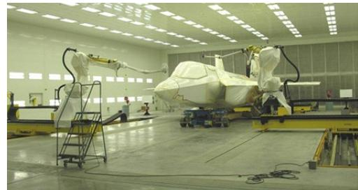
Pictured here is a robotic painting work cell. A new lightweight coating system eliminates one layer of paint from the traditional system resulting in an overall aircraft weight reduction and over 50% reduction in the paint/paint-removal waste stream.
