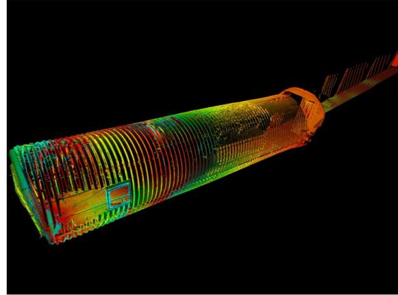
**Point Cloud of Alert Facility Tunnel:** A digital point cloud of one of the egress tunnels of Building 291, Mountain Home AFB. The building is historically significant as a Cold War era strategic bomber alert facility. Recorded using state of the art laser based technology, these data sets provide the installation with precise documentation at minimal cost.
