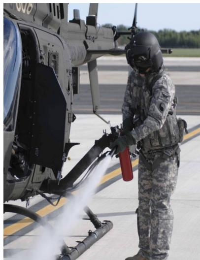
**Discharge Demonstration:** 5th Percentile Aviator demonstrating a successful discharge operation and function of the non-ODS HHFE.
