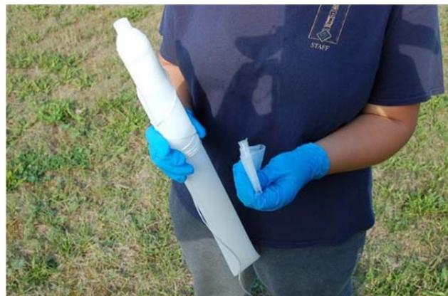
Less waste is generated using a passive diffusion bag (in left hand) than either a disposable bailer or disposable tubing associated with using a pump.
