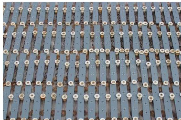
*Outdoor exposure test coupons for seven hexavalent chromium-free surface paint systems are set up for long exposure tests. Tests are conducted under high humidity, rainfall, and salt conditions in Daytona, Florida.*
