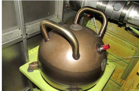
*The KC-46A will be the first airliner/transport-type airframe in the world delivered with an FAA-certified non-halon engine and APU fire suppression system.*
