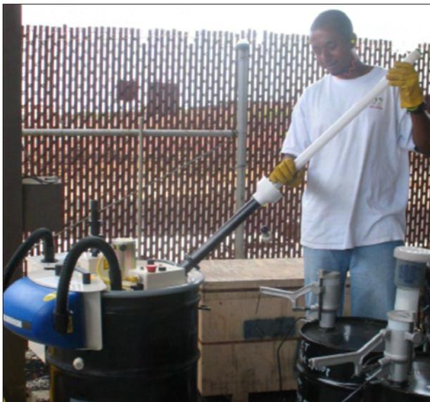
Aerosol Can Puncturing and Fluorescent Lamp Crusher
