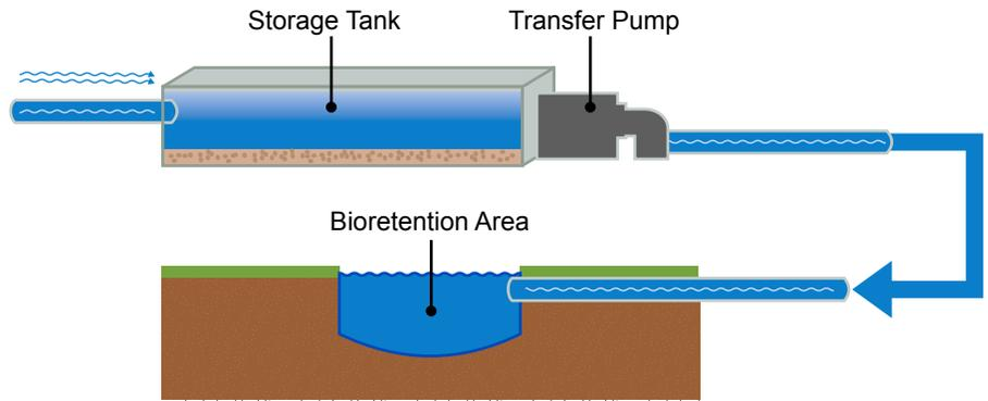
System diagram of the prototype installed at the Perry Center: stormwater flows into a storage tank where debris are settled. A pump transfers water based on the level to a downstream bioretention cell.
