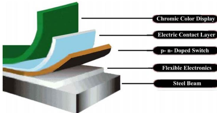
**Figure 4.6 Multifunctional Anti-Corrosion Coating**
