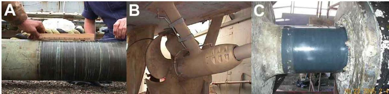
**Figure 4.7 USS Ardent Propulsion Shaft Coating**
