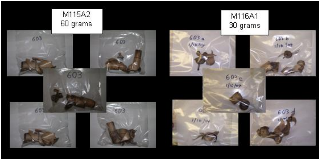
Figure 15: Fragmented housing bodies for 603 mix in M115A2 and M116A1
