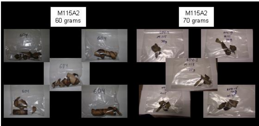
Figure 16: Fragmented housing bodies for 604 mix in M115A2
