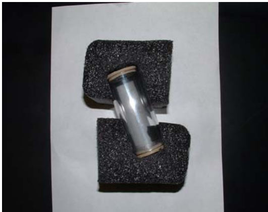
Figure 5: Clear polycarbonate tube model for mixing study
