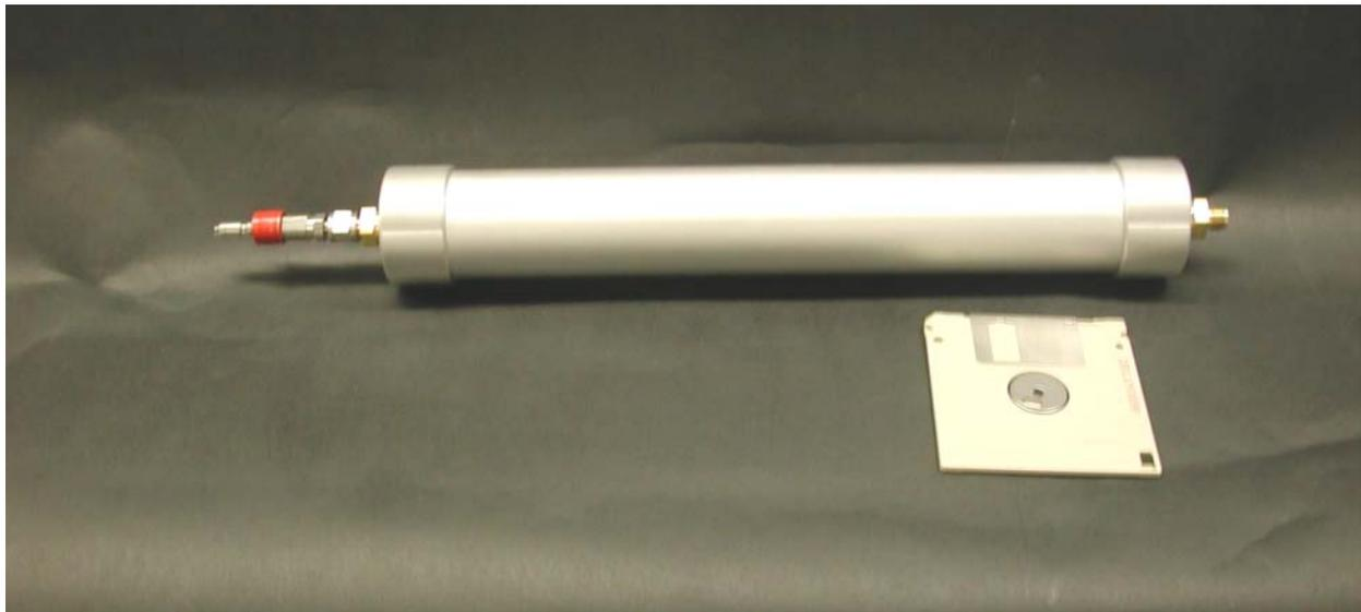
**Figure 5-7 An example of a possible adsorbents cartridge design for capturing lost  $\text{SF}_6$  during the sampling process**
