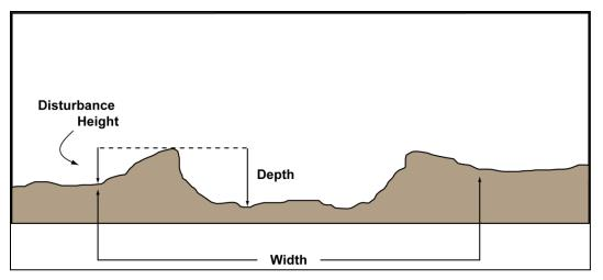
Figure 3-2. Rut Measurements.
