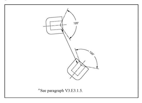
Figure V3.E3.F3. ECM Orientation Effects on IMD: Side-to-Side Orientation<sup>a</sup>
