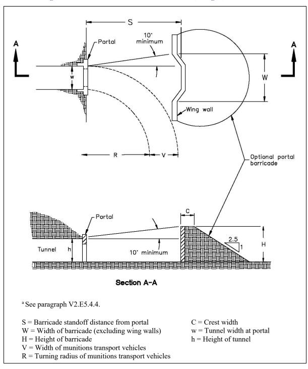
Figure V2.E5.F2. Portal Barricade Location, Height, and Width<sup>a</sup>
