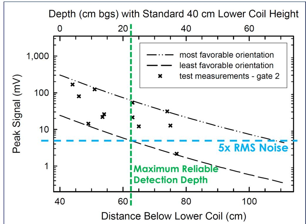
Sensor Response Curve - EM61-MK2 response curve for small Industry Standard Object (ISO; 1"x4" steel pipe nipple).
