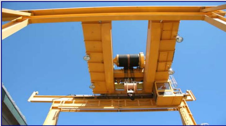
200-ton Ederer overhead bridge crane before it was outfitted with self-retractable lifeline fall protection devices. Riggers had to climb out onto the component to attach rigging device to the crane hook.
