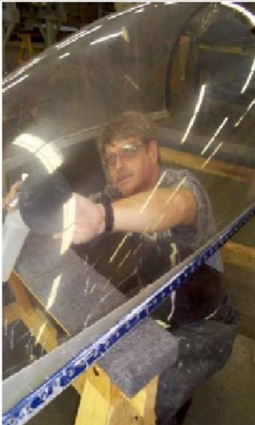
Mechanic having difficulty working on underside of canopy before ergonomic improvements
