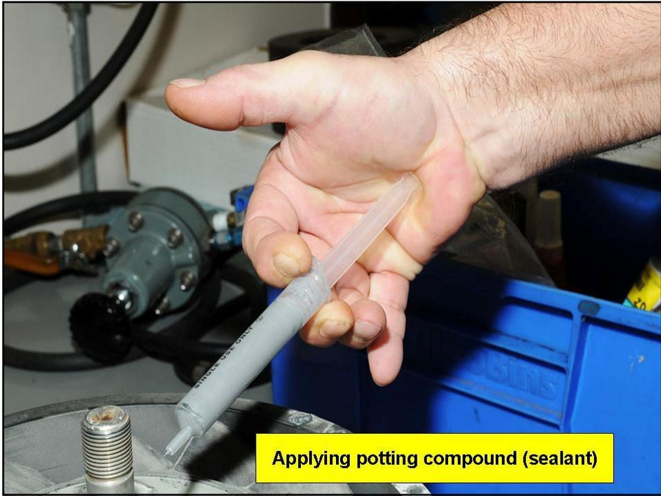
Applying potting compound (sealant)
