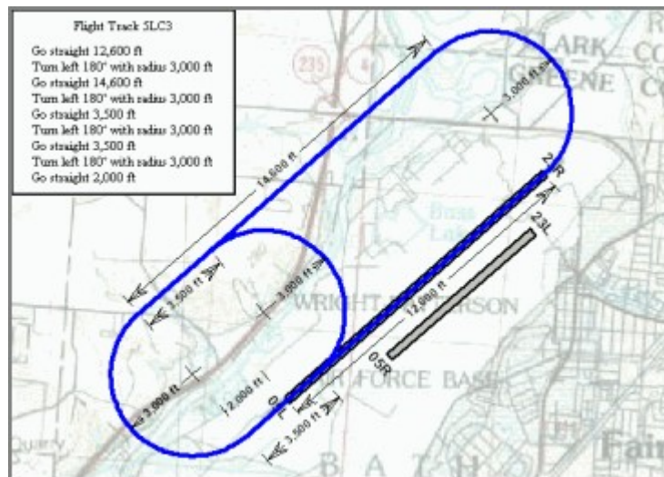
Sample flight track map, with flight track table in upper-left corner
