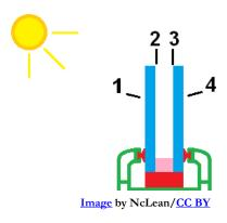
Fig 1: Window Surface Diagram – Depicts surface #1 (outside facing pane), surface #2 (inside of outside facing pane), surface #3 (inside of inside facing pane and) and surface #4 (inside facing pane).
