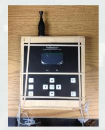
Pettersson bat detector with balsa wood box, hanging attachments, and Li-lon battery
