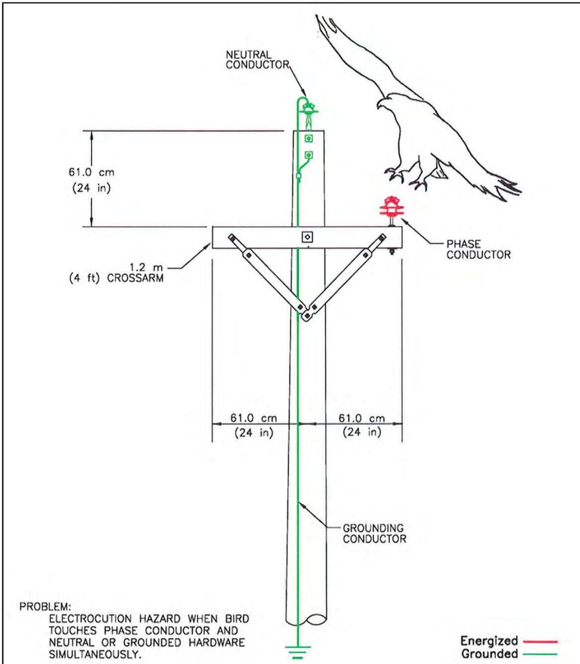
Figure A-3. Problem single-phase configuration with crossarm and overhead neutral.
