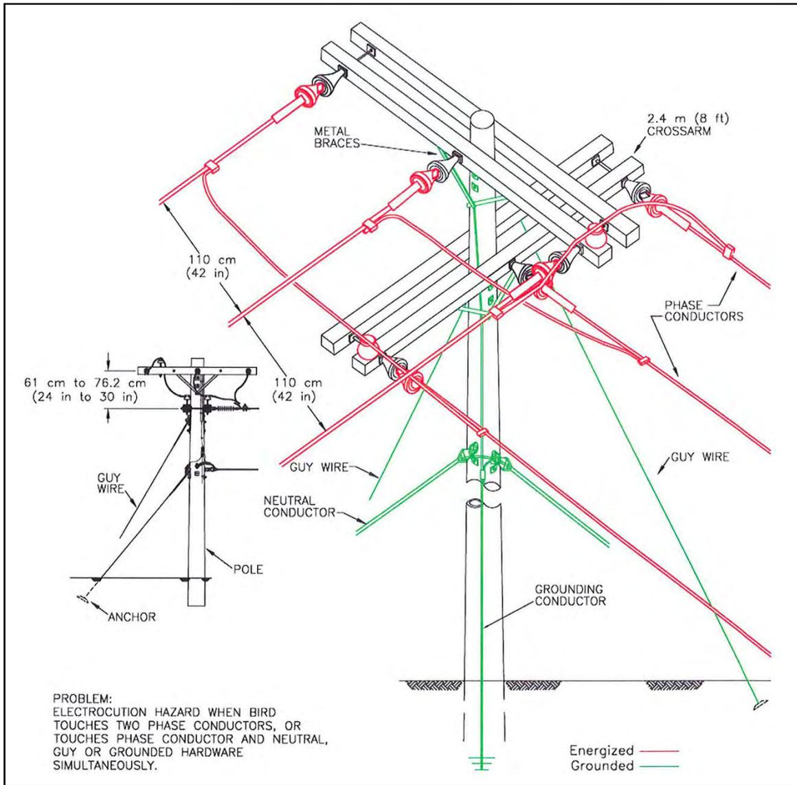
Figure A-17. Problem three-phase distribution corner configuration.
