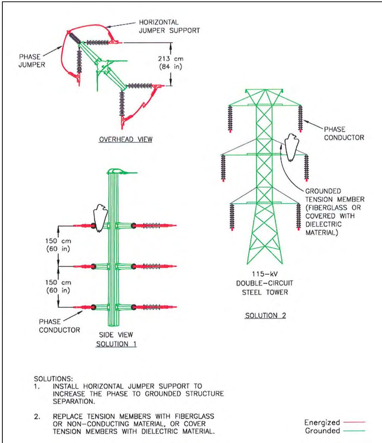
Figure A-38. Solutions for transmission design.
