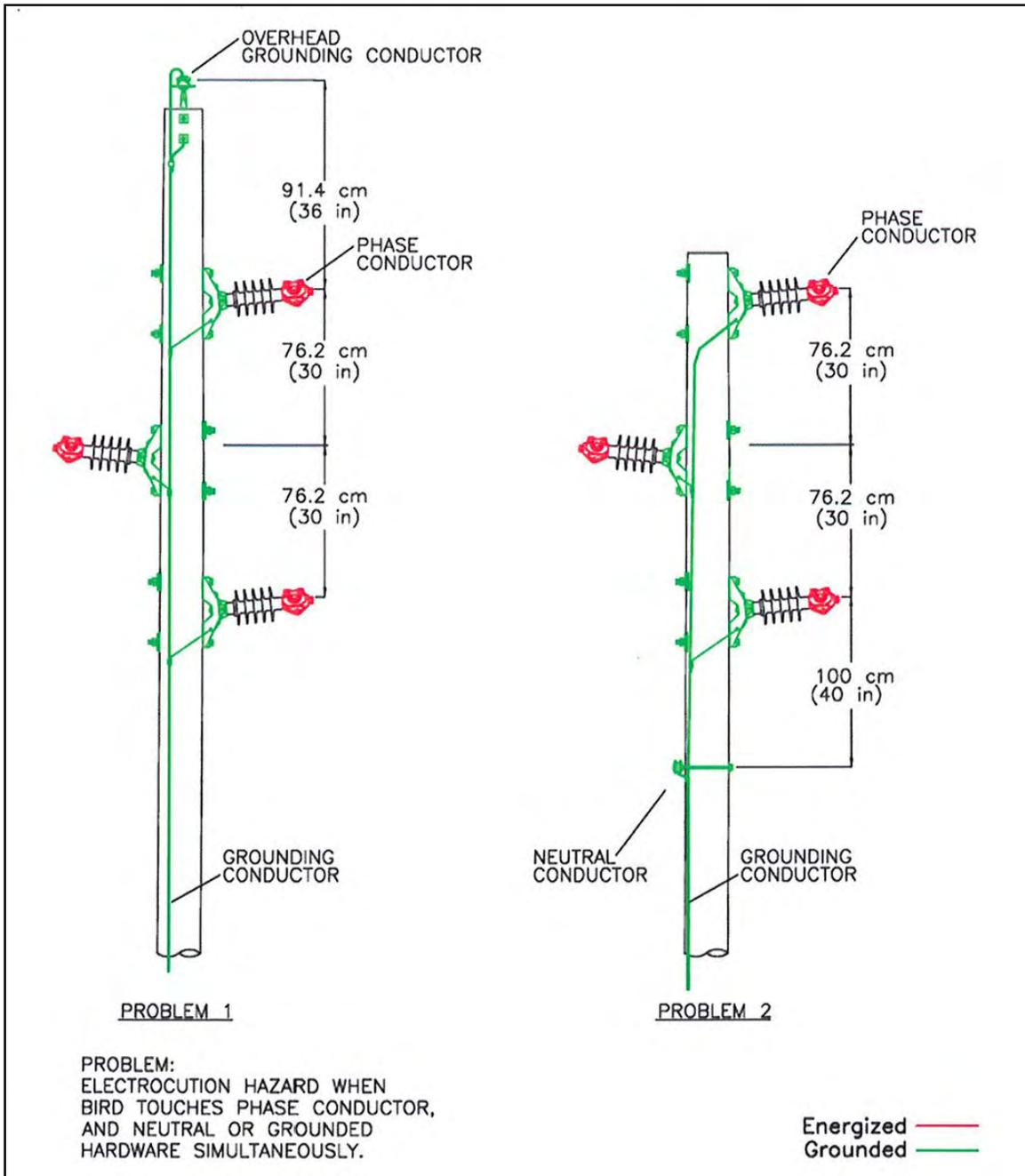
Figure A-15. Problem distribution horizontal post insulator designs.
