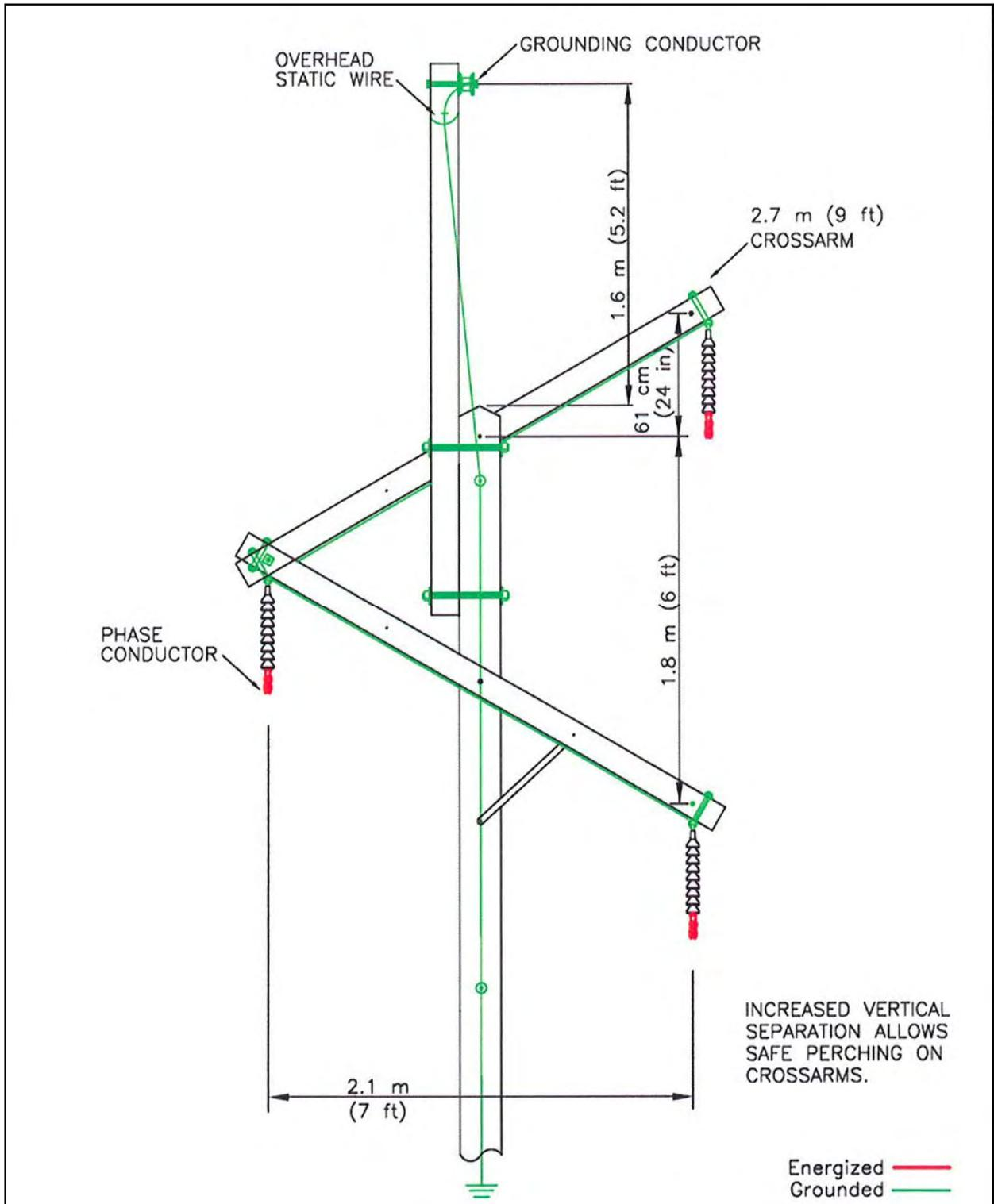
Figure A-33. Avian-safe wishbone construction.
