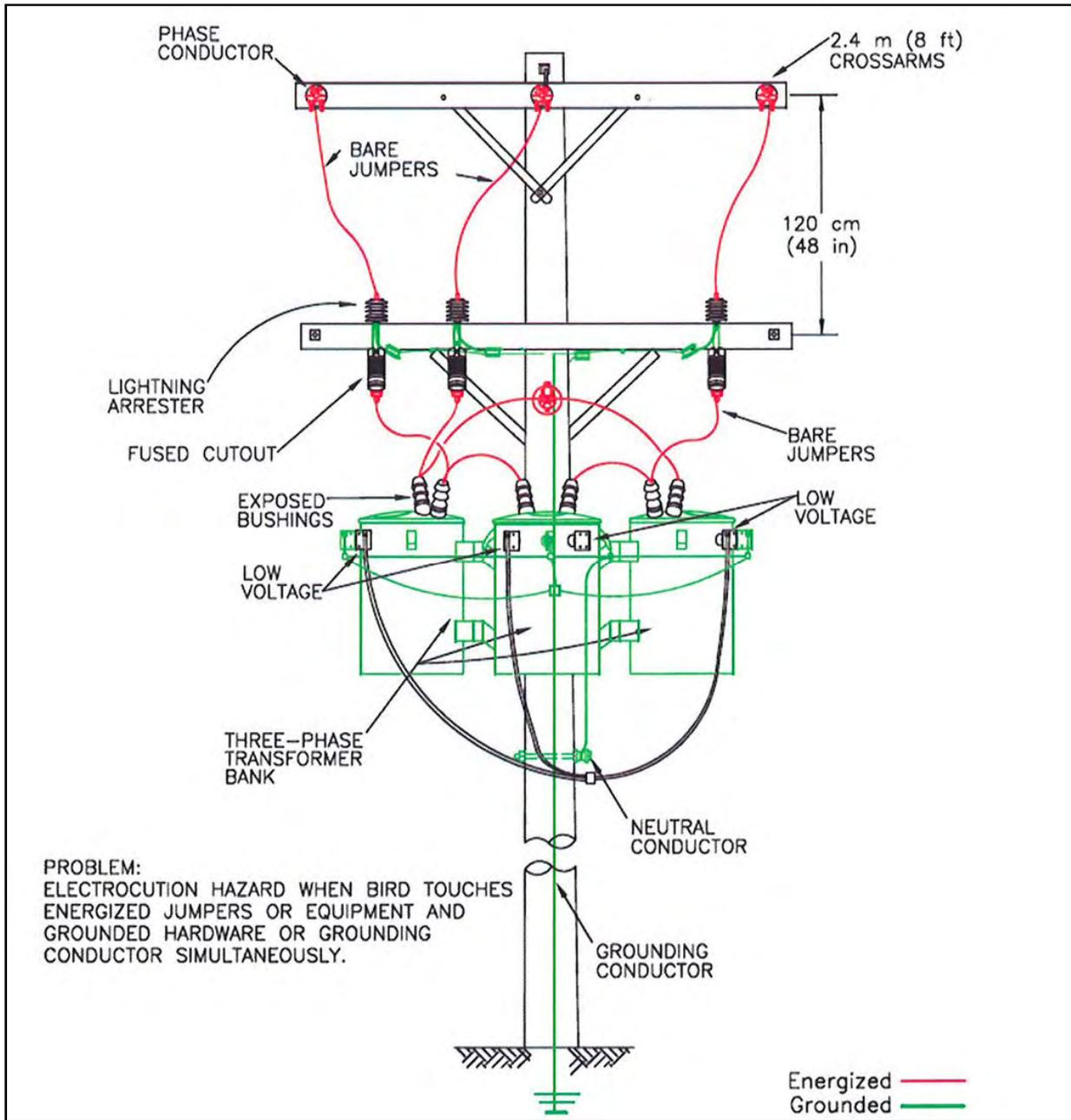
Figure A-39. Problem three-phase transformer bank.
