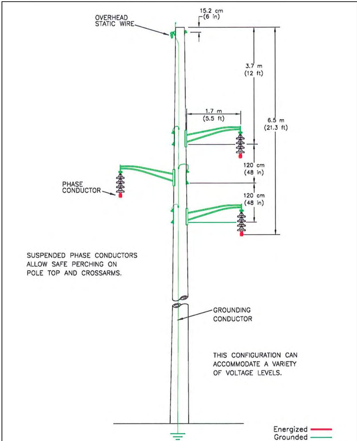
Figure A-34. Avian-safe suspension configuration.
