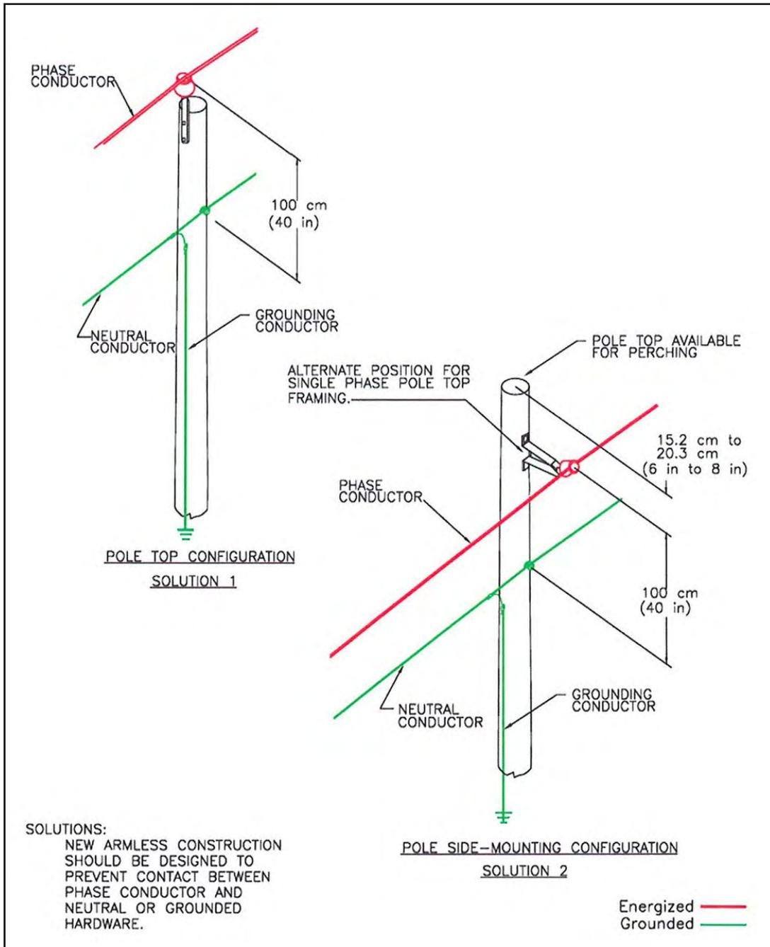
Figure A-5. Single-phase avian-safe new construction.
