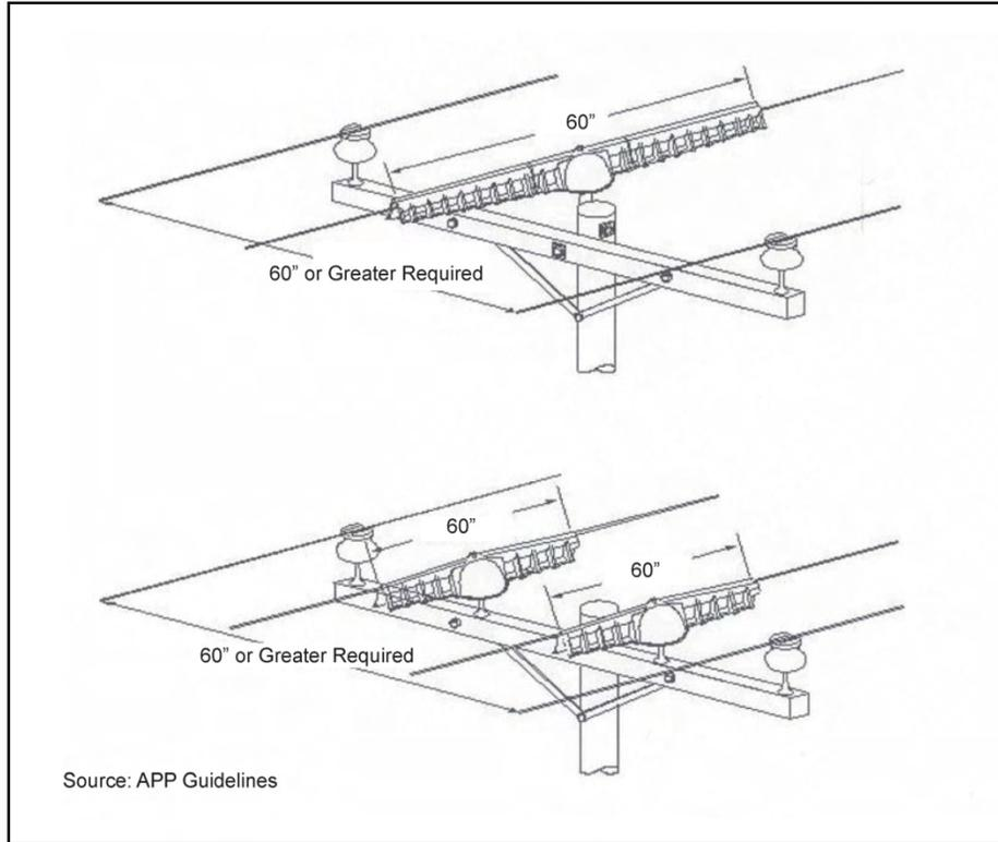
**Figure 21. Avian-safe Structure with Perch Covers**
