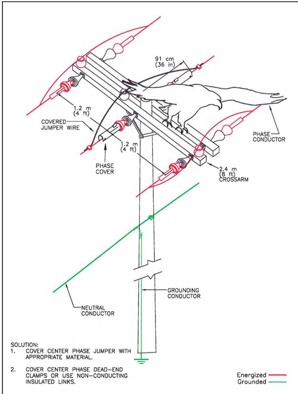
Figure A-11. Solution for three-phase double dead-end with exposed jumper wires.
