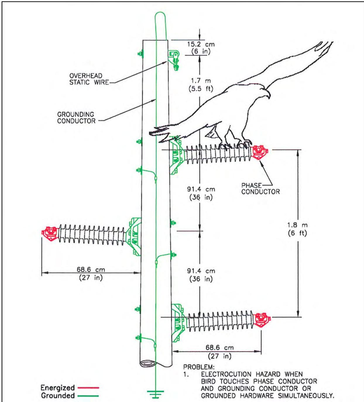
Figure A-29. Problem 69-kV post insulator design.
