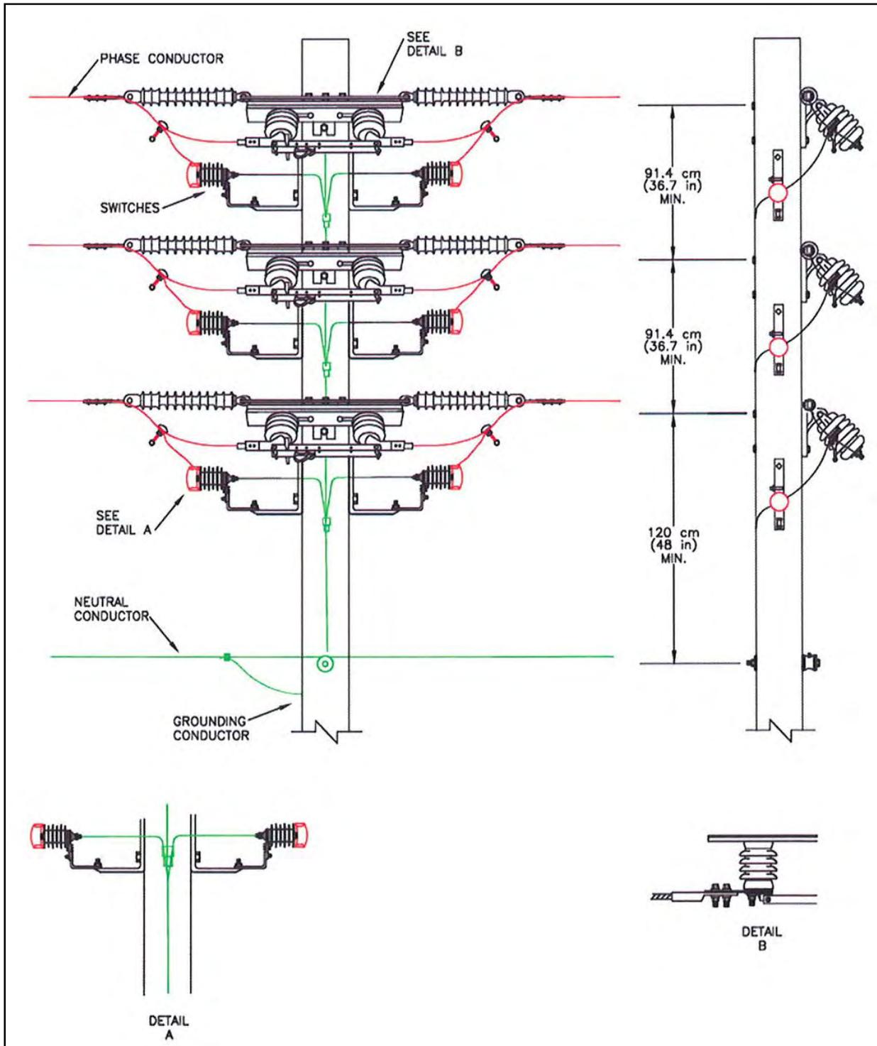
Figure A-45. Pole-mounted switches.
