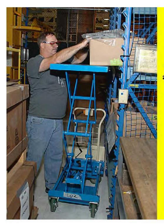
Mobile handling scissor lift table with battery lift operation that enables the operator to place the load at a convenient working height.
