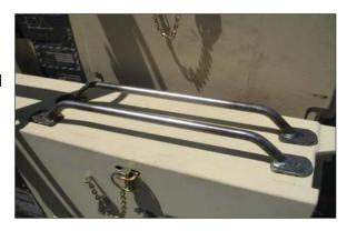
Maintenance personnel can now safely use three-point contact when climbing up to conduct service on the PLS.
