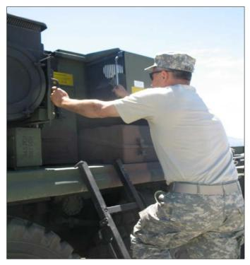
The newly designed safety handle mitigates ergonomic risk factors. It balances body load forces by establishing solid three-point contact when climbing on a PLS to conduct maintenance checks.
