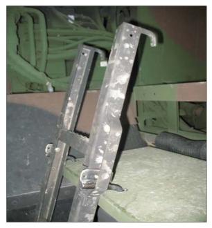
After conducting the JHA, the teams came up with a low-cost (less than \$10 for material) engineering control. A simple, but effective ladder modification was the answer to mitigate the hazard. The teams designed and added two more hooks and drilled two holes so the existing ladder could be used in another area.
