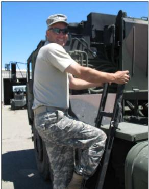
A 423rd soldier demonstrates the existing PLS ladder that was modified to access the rear service platform. This new modification will help prevent climbing, falling, and ergonomic injuries on the PLS.
