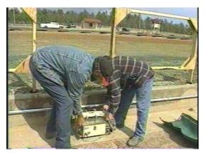
Changing target mechanism and lowering target.
