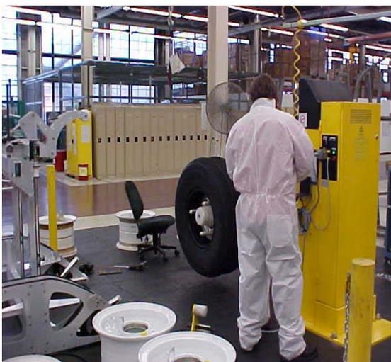
Mr. Rew adjusts controls on Ergo Tech Robot to maneuver tire to an ergonomic work position.
