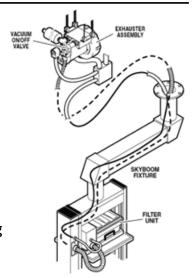
Sky Vacuum captures and removes potentially harmful laser and electro-surgical smoke particles from breathing space of OR team.
