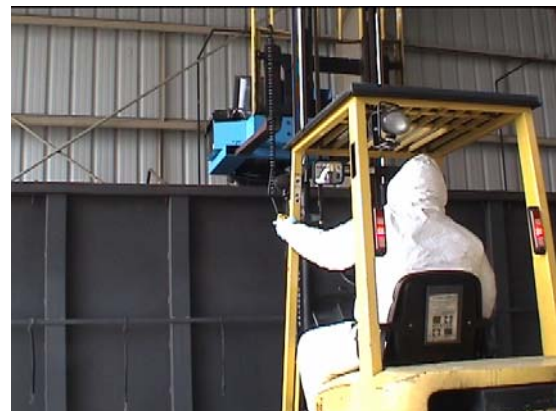
Dump draining using an electric drum dumper.
