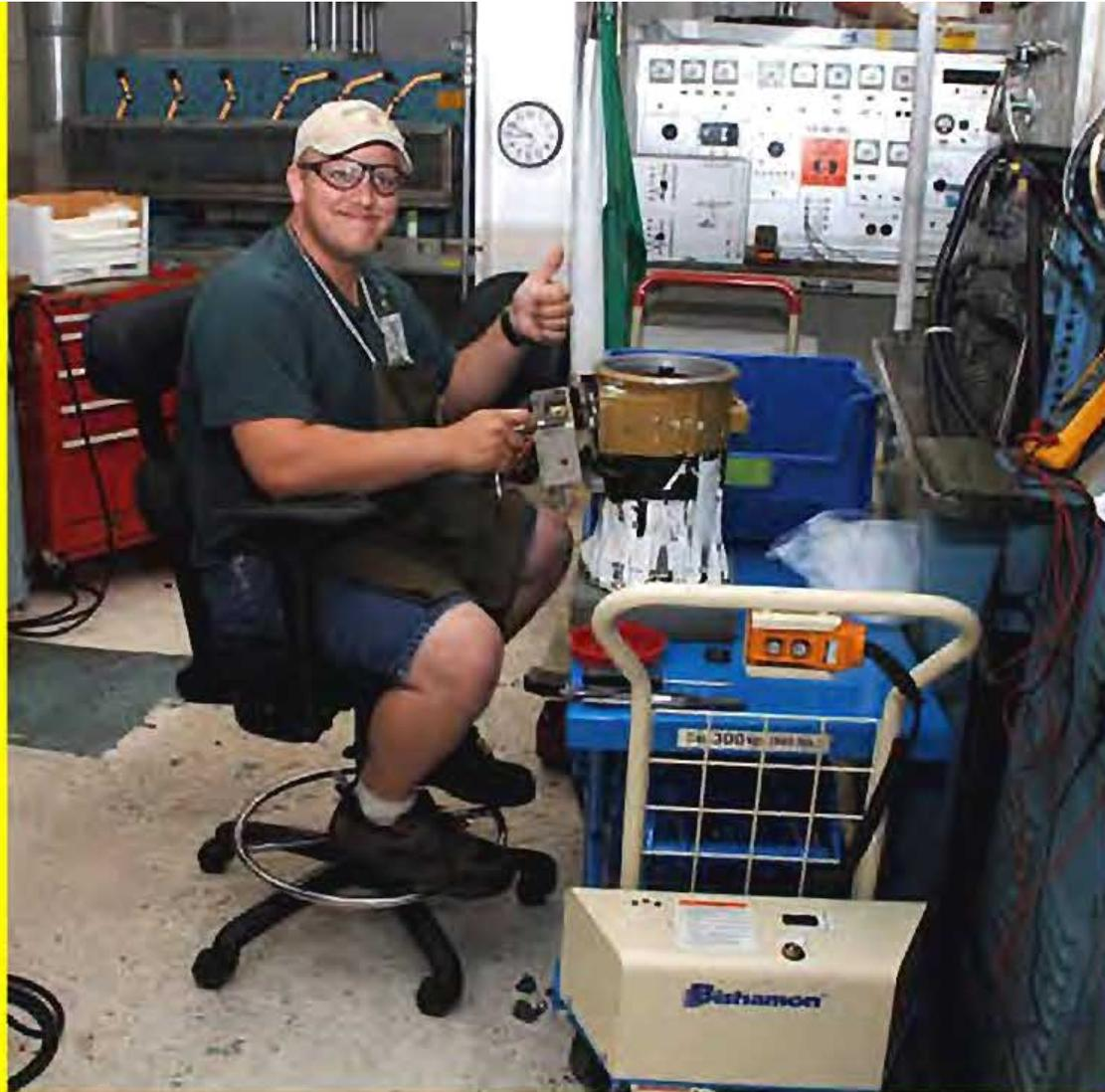
**Mobile handling scissor lift table with battery lift operation that enables the operator to place the load at a convenient working height. When completed the generator can be lifted into the paint booth using the scissor lift.**
