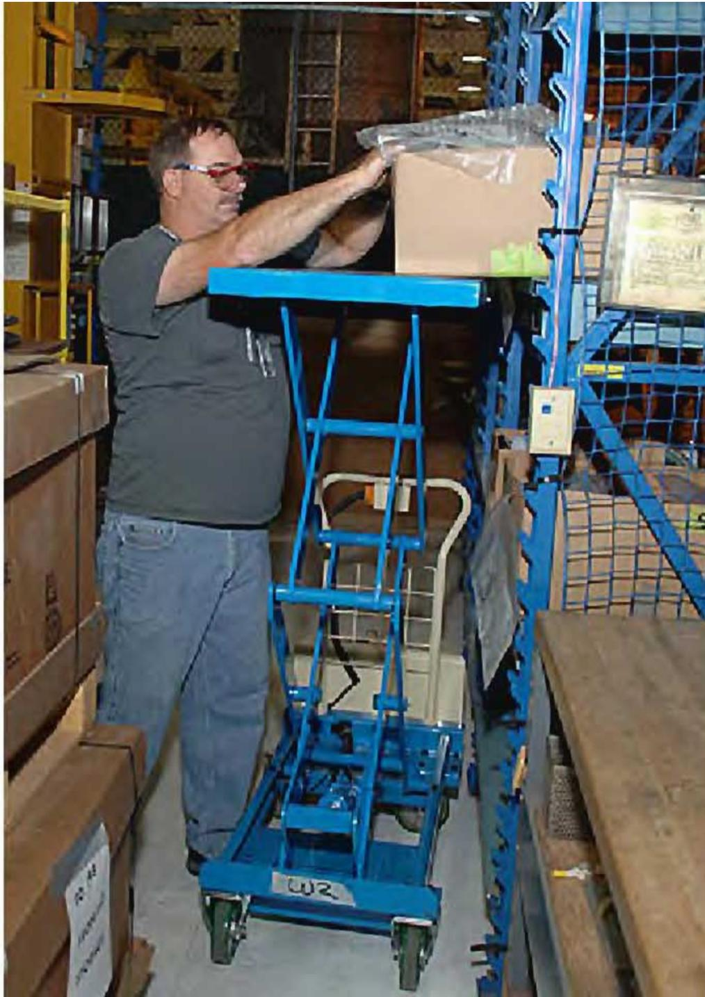
**Mobile handling scissor lift table with battery lift operation that enables the operator to place the load at a convenient working height.**
