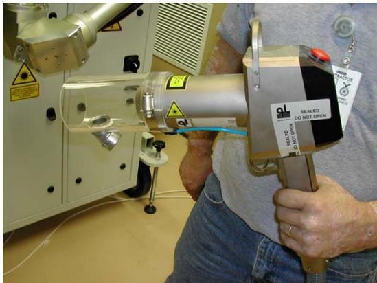
The operator added a nozzle end to the 40-watt handheld laser to serve as a capture vent. The ventilation hose is not attached.
