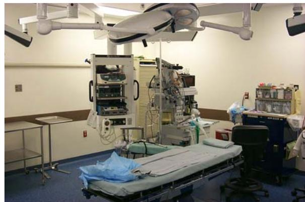
System of ceiling-mounted boom racks and flat-panel video displays located on suspended, swiveling racks reduces clutter in OR and allows surgical team to work in neutral postures.
