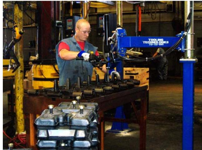
Providing a special design tool developed by a tool manufacturer allows this worker to maintain a neutral work posture, exert less force, and meet production requirements.
