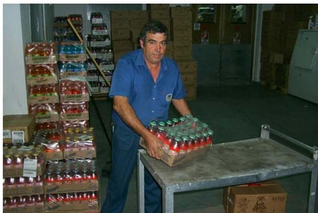
Ergonomically designed material transport carts lessen the force needed for manual material movement duties in various supply department warehouses, the base hazardous material center, etc.
