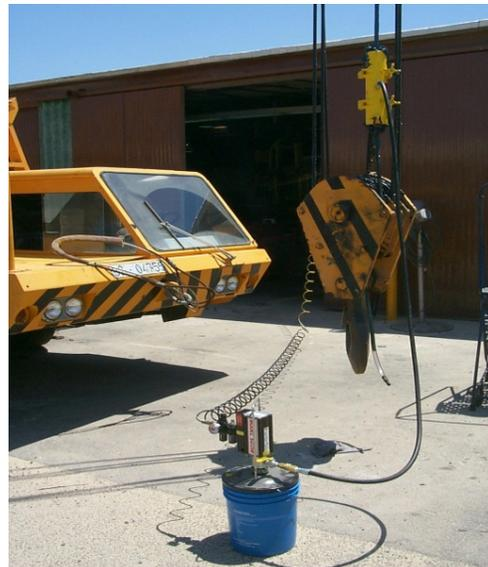
Automated crane cable lubrication and cleaning system allows a single worker to clean and lubricate these VERY long and heavy cables in a seated posture. Before this ergo improvement, cables were cleaned and lubricated by hand literally foot-by-foot by TWO workers standing on their feet all shift.
