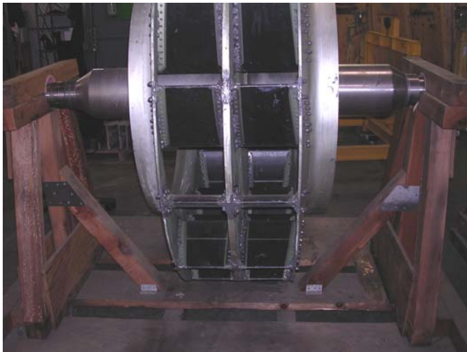
Photo 1: Fan on wooden fixture
