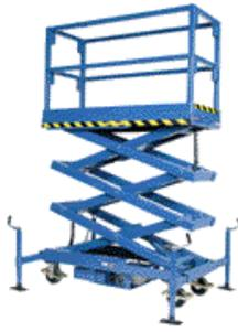
New Dominion produced a price quote of \$60,400 for equipment, installation, and shipping of a 4 level lift with 2,000 lb. capacity and a 26' travel distance.
