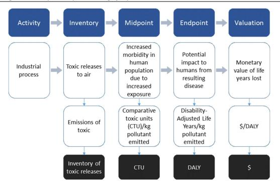
Figure 13. Example Cause-Effect Chain for Estimating Impacts from Toxic Release to Air
