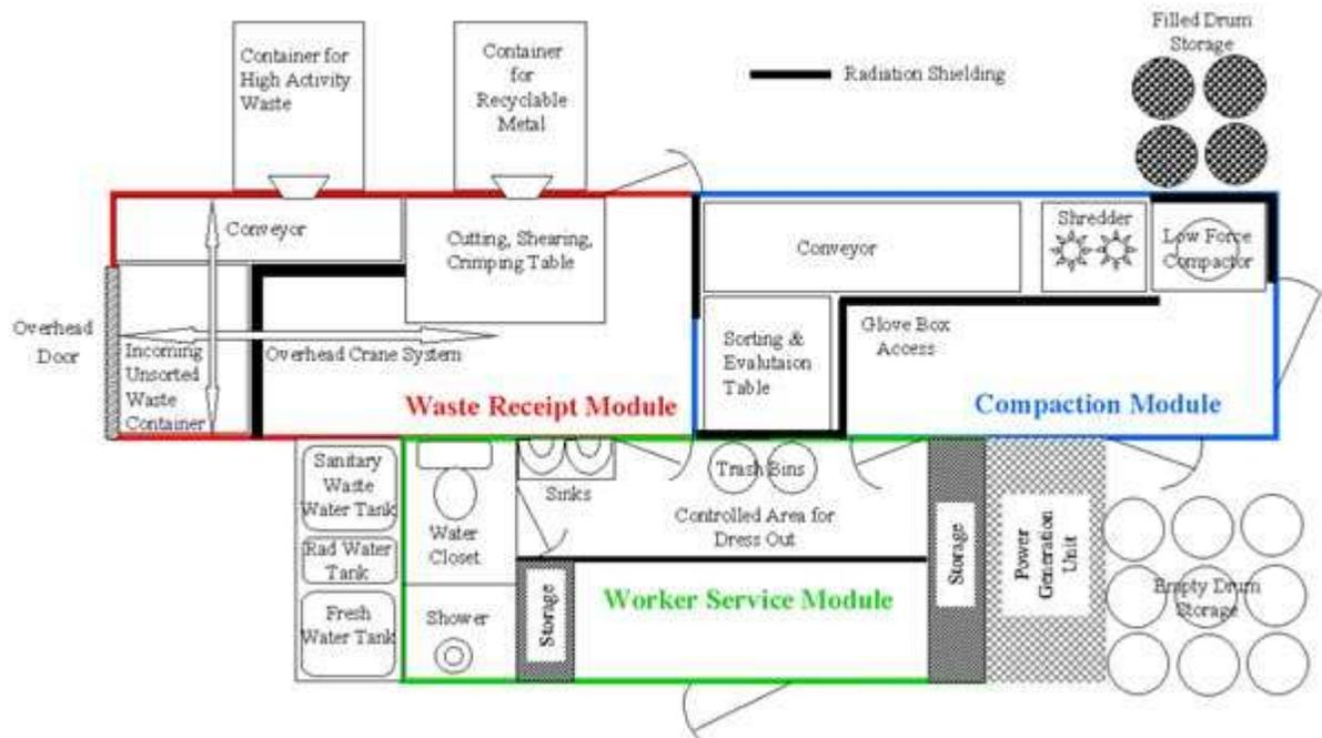
**Figure 3.** Modules of Mobile Pretreatment Facility
