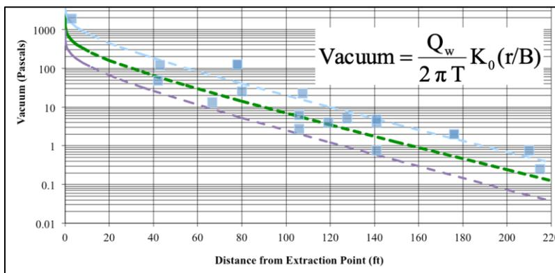
Figure 2b: Vacuum versus Distance Data and Steady-State Model Analysis Using a Spreadsheet
