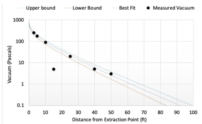
**Figure 4: Example of Lower-than-Expected Vacuum at a Probe Near a Preferential Pathway**
