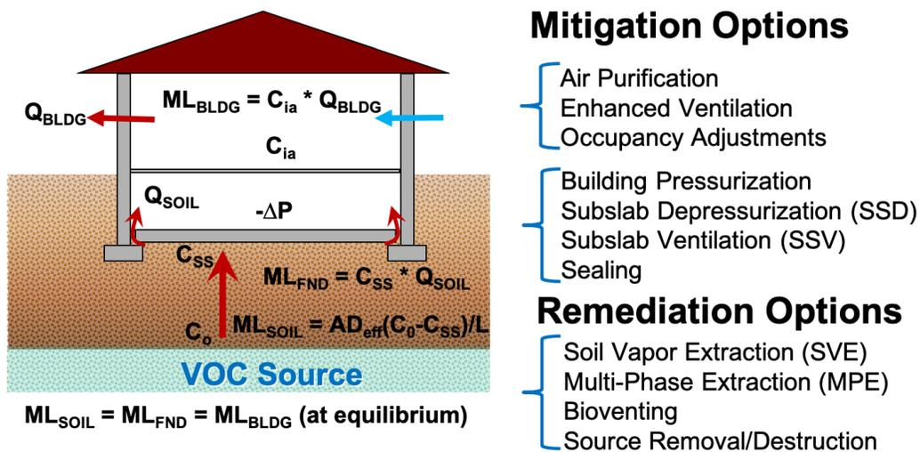
**Figure 1: Conceptualization of VOC Mass Loadings with Corresponding Options for Mitigation and Remediation**
