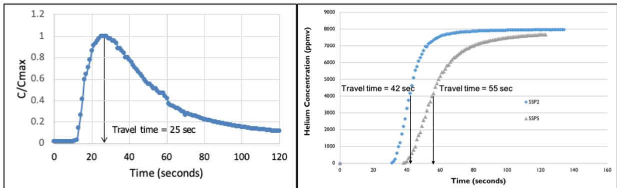
**Figure 3: Tracer Test Plots for Inter-Well Test (3a, left) and Flood Test (3b, right)**
