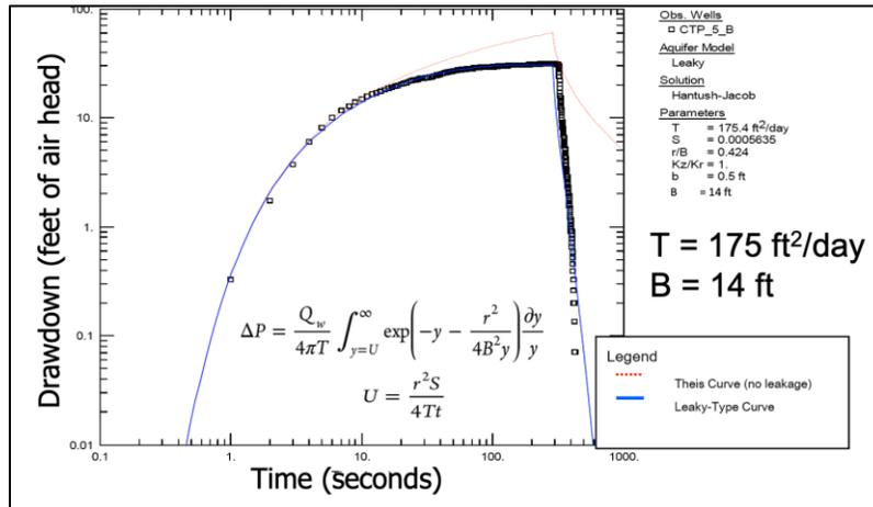
Figure 2a: Vacuum versus Time Data and Transient Model Analysis using AQTESOLV® Software
