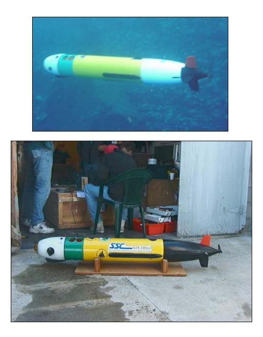
Photos 3 & 4: AUV developed for the Office of Naval Research funded Chemical Sensing in the Marine Environment program.
