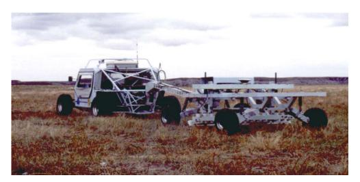
Figure 3b. Multiple Towed Array Detection System (MTADS)
