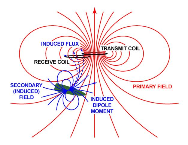
Figure D-10. Electromagnetic Induction (EMI)
