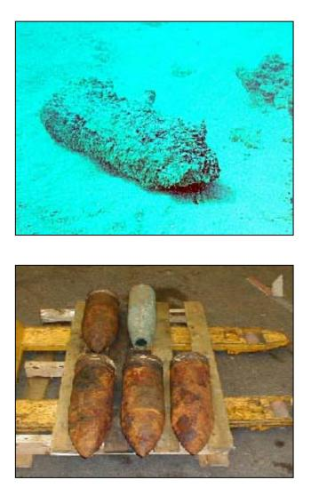
Photos 1 & 2: WW-I and WW-II era coastal defense 6-inch projectile underwater south of Oahu, Hawaii (*top*) and recovered shells from the same area with encrusting growth removed (*bottom*).
