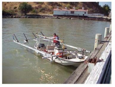
Photo 5. Alpha Geoscience/SONTEC mounted AGS-2 Magnetometer.
