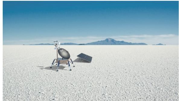
In-situ mockup of Picogrid terminal unit and example sensor suite.
