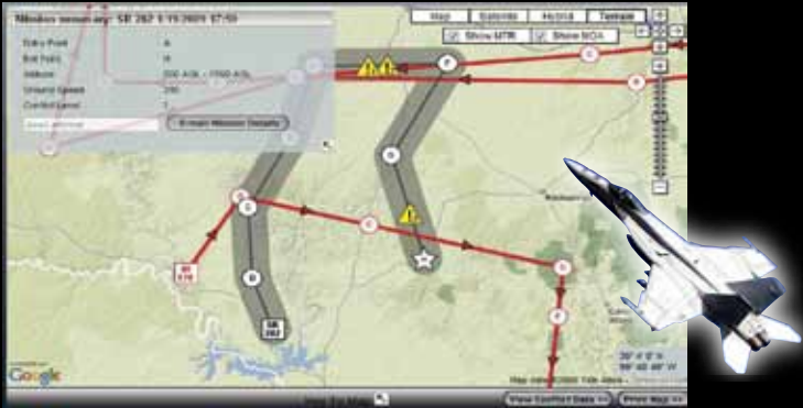
JLLDT interface clearly warns pilots of potential conflict on their scheduled missions. It includes yellow warning triangle icons on the map and in a summary box with details. The tabular interface also displays the mission conflict data in a very easy to use user interface.
