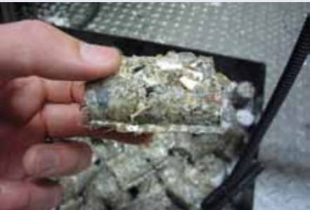
During a July 2011 demonstration, the OFWEC III technology reduced the weight of incoming waste by 90% and offset up to 34% of the diesel fuel used to operate a Tactical Quiet Generator.
